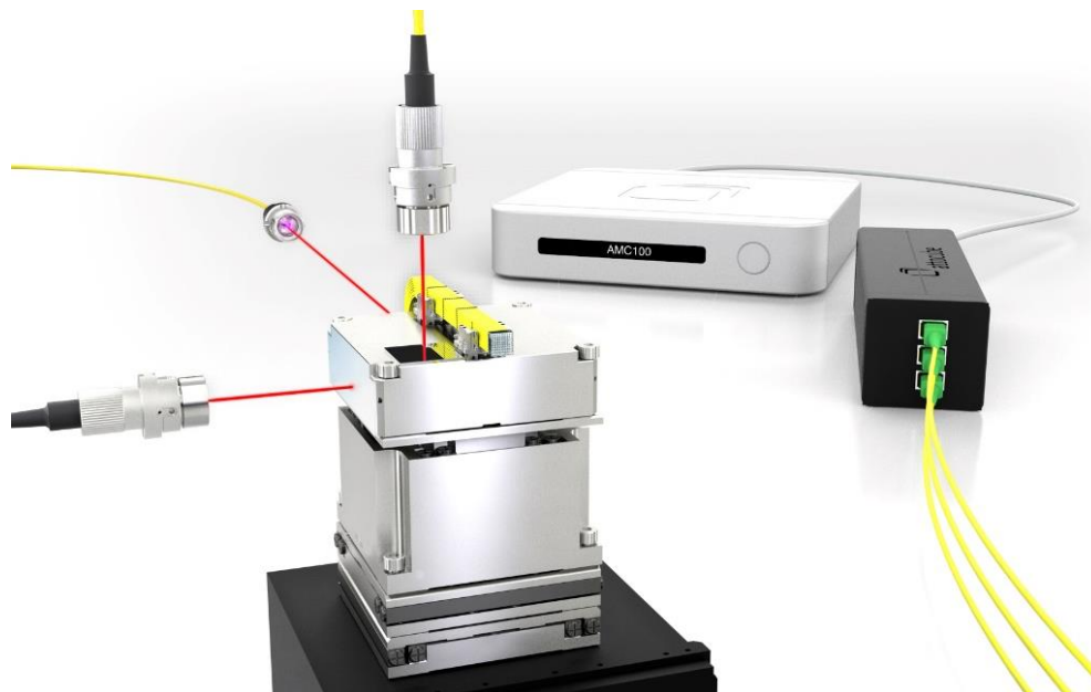
Figure 1: Interferometric closed loop control of an XYZ positioner stack using the AMC100 and the IDS3010. The fiber array and a mirror block are mounted on the top positioner. The 3 miniaturized sensor heads measure the XYZ displacement close to the point of interest (= fiber array).
